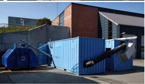
100 kW combined steamdryer and pyrolysis
